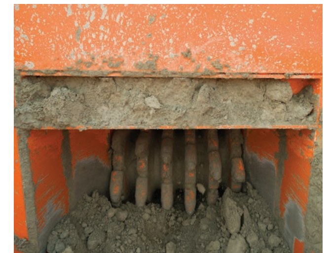
A powerful rotary pick breaker reduces material to a consistent size easily handled by conveyor belts and secondary crushing operations. The carbide-tipped picks on the breaker shafts are designed to interlace with solid steel alloy flights to maintain a consistent product size.
