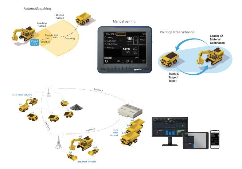
The Smart Quarry Site Mesh Network is made up of a collection of wireless networking devices running Smart Quarry Site mesh networking software.
