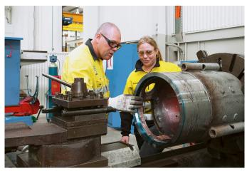
A Fitter and Turner will learn the trade to fabricate industrial tools, components and products from metal. Working to a set of specifications, operating tools and machines to grind, mill and shape raw materials into the specified form, then assembling the final.
