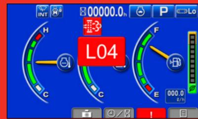
KDPF system failure – manual stationary regeneration is disabled. Stop the engine IMMEDIATELY. The KDPF system requires inspection and maintenance. Contact your Komatsu distributor for assistance and service.
