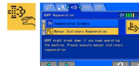
**Effect on Operation:** YES, the machine must be parked in the correct idle position and cannot be operated till MSR is complete.
