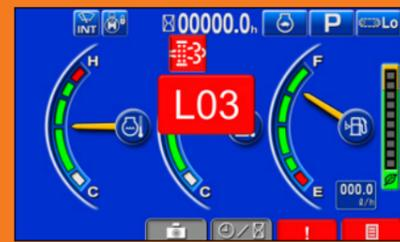
Manual Stationary Regeneration Required. Stop current work, move the machine to a safe place, park it in the correct idle position and perform a manual stationary regeneration.
