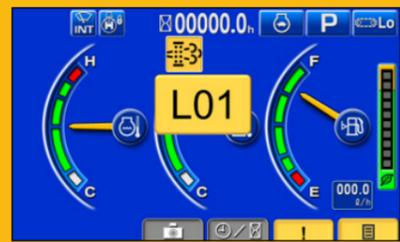
Manual Stationary Regeneration Request. When current work is completed, move the machine to a safe place, park it in the correct idle position perform a manual stationary regeneration.
