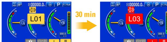
If this request is ignored by the operator for 30 minutes, the caution level is changed to L03 and the engine will begin to derate. The regeneration must be run immediately so that the exhaust temperatures can be raised safely.
