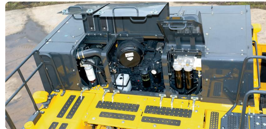
Easy access to filters on the front side of the engine hood.
