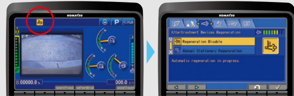
Aftertreatment device regeneration screen
