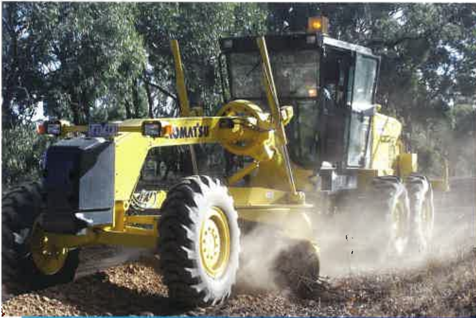
Mitchell Shire's recently delivered GD555-3 grader has plenty of pushing power with its unique dual transmission system.
