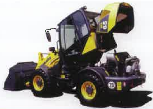
The WA65-5 has a unique tilt-up cab feature, giving rapid and easy access to all major components.
