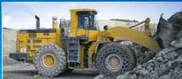
WA600-3 fitted with K VX G.E.T. system
