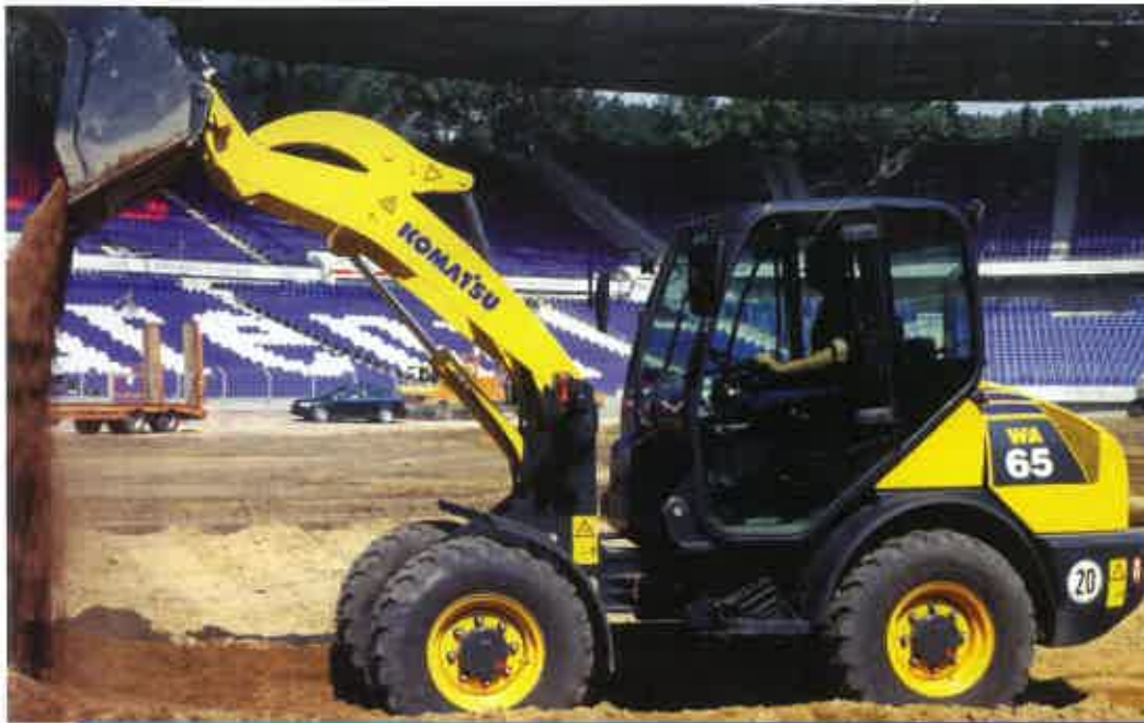
Komatsu's new WA65-5 loader has been designed for quick and easy transport between jobsites. It features hydrostatic drive and a Tier II-compliant engine.
