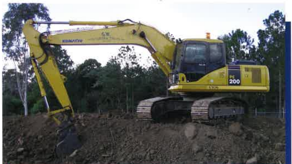
One of Queensland-based GW Civil's two PC200-7 excavators; these have proved far more fuel-efficient than their Dash 6 predecessors.
