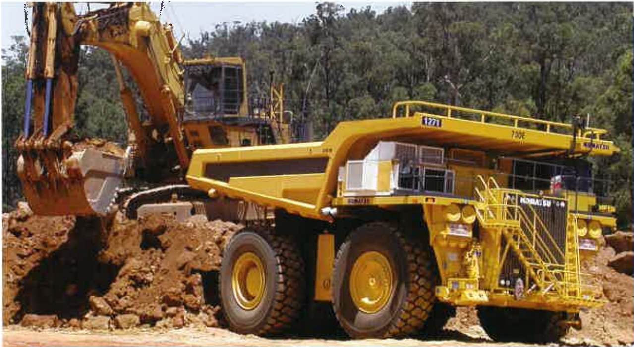
One of Alcoa's recently delivered fleet of 12 Komatsu 730E dump trucks, purchased with the aim of achieving a "step change" in lower haulage and operating costs.
