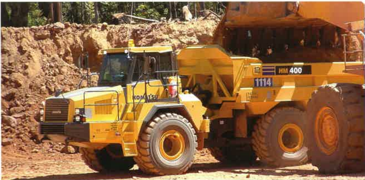
Alcoa is using Komatsu's AcuMine HaulCheck system to allow it to run larger trucks in the same-width haulroads.
