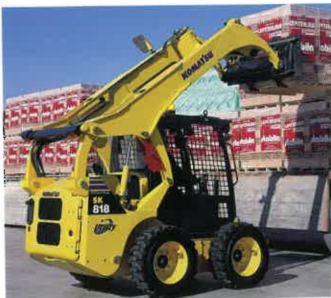
The SK818-5 has a vertical lift geometry, allowing greater lift at maximum height.
