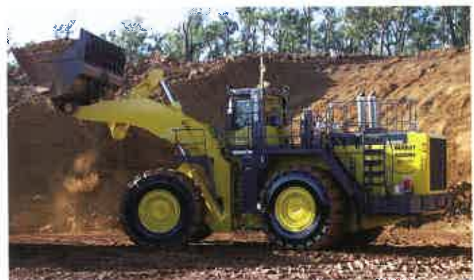
Worsley Alumina's silenced WA900-3 loader works at only 108 dBA.
