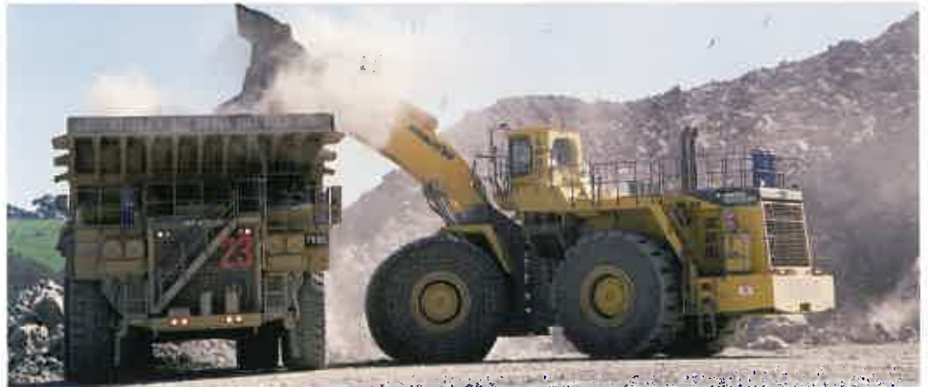
Komatsu's WA1200-3 loading a 230 tonne dump truck at Cadia Valley gold mine in NSW.
