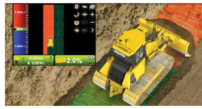
No grade checks required, removing the need for people to work around mobile equipment.
