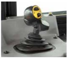
Palm Command Control System (PCCS) with automatic/ manual blade control button
