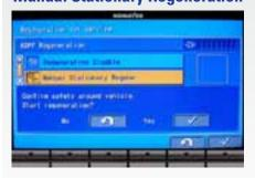
Under most conditions, active regeneration will occur automatically with no effect on machine operation. In case the operator needs to disable active regeneration or initiate a manual stationary regeneration, such as in high-combustible applications, this can be easily accomplished through the monitor panel. The soot level indicator identifies how much soot is trapped in the KDPF.
