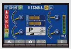
The LCD colour monitor panel provides the operator with the status of the KDPF regeneration without interfering with daily operation. When the machine initiates active generation, an icon will notify the operator.
