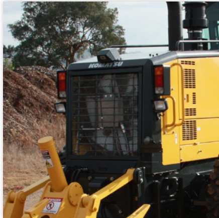
Easy radiator cleaning with reverse fan
