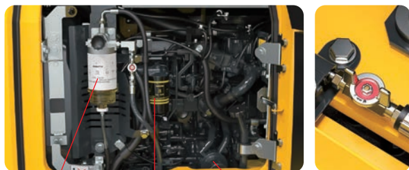
Fuel pre-filter (With water separator) High efficiency fuel filter Engine oil filter Fuel drain valve
