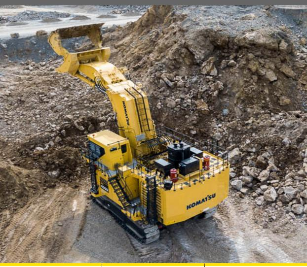
ENGINE POWER 1400 kW / 1875 HP @ 1800 rpm **OPERATING WEIGHT** 393 – 409 tonnes / 866,400 -901,700 lb SHOVEL CAPACITY 22 m<sup>3</sup> 29 yd<sup>3</sup> SAE 2:1 heaped
