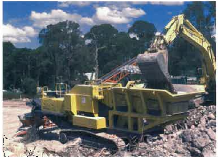
A BR500JG Mobile Crusher similar to the one purchased by Davis Earthmoving
