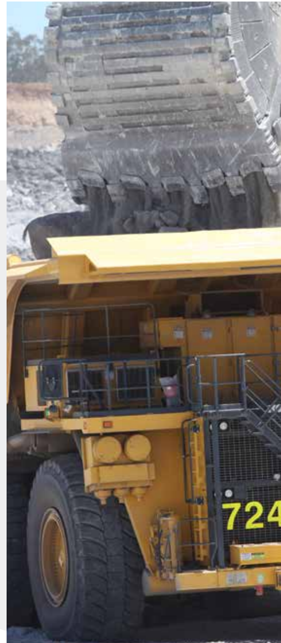
Overburden haulage at Boggabri Coal is spearheaded by 17 Komatsu 930E trucks powered by Cummins QSK60 engines rated at 2700 hp.
