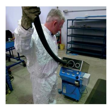
Specialised cleaning techniques to ensure the hose assembly is contaminant-free and all assemblies are individually bagged and capped to prevent damage and contamination of the assembly. All assemblies are clearly tagged to make re-ordering your hose simple and easy. Komatsu Engineering Standard (KES) assembly techniques ensures traceability of products and components that are used in the assembly process.
