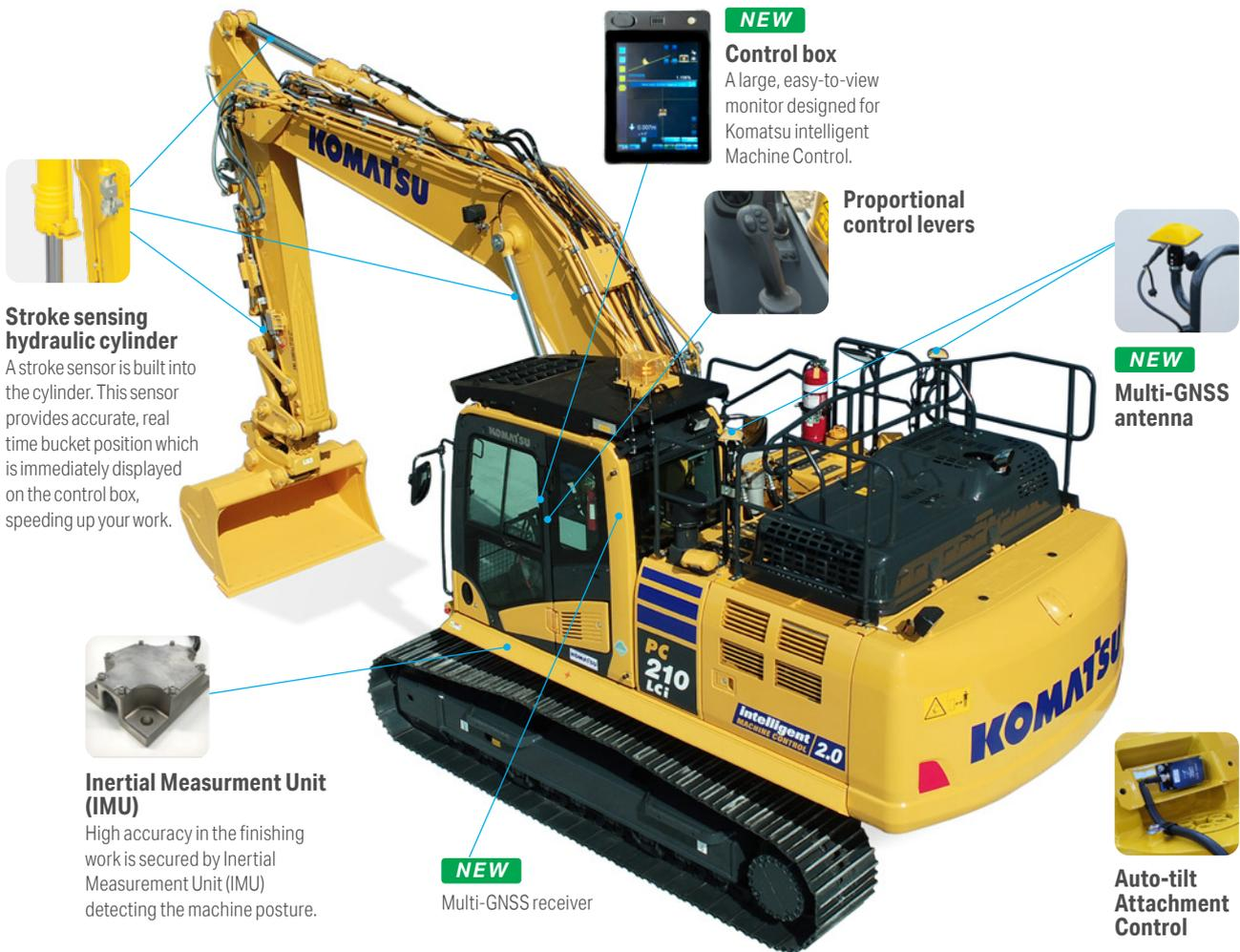
**Stroke sensing hydraulic cylinder**
