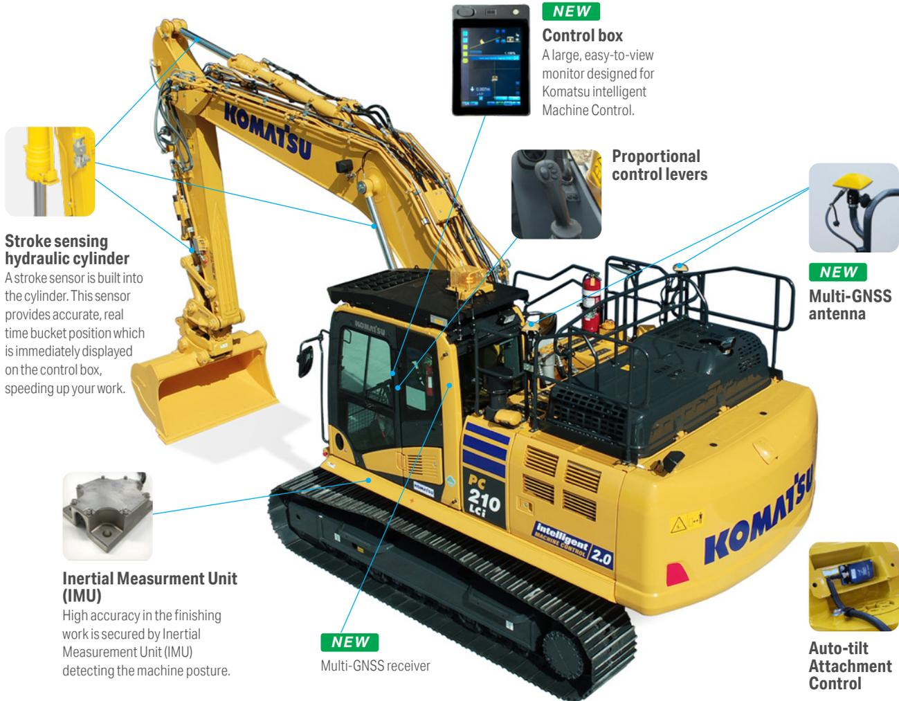
**Stroke sensing hydraulic cylinder**
