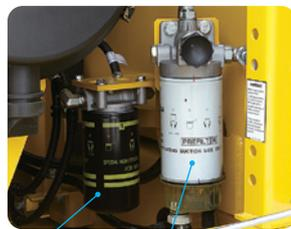
High efficiency fuel filter      Fuel pre-filter (with water separator)
