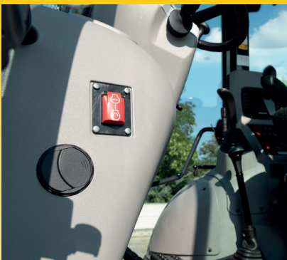
Secondary engine shut down switch
