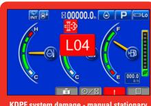
KDPF system damage - manual stationary regeneration is disabled \_\_\_\_\_
