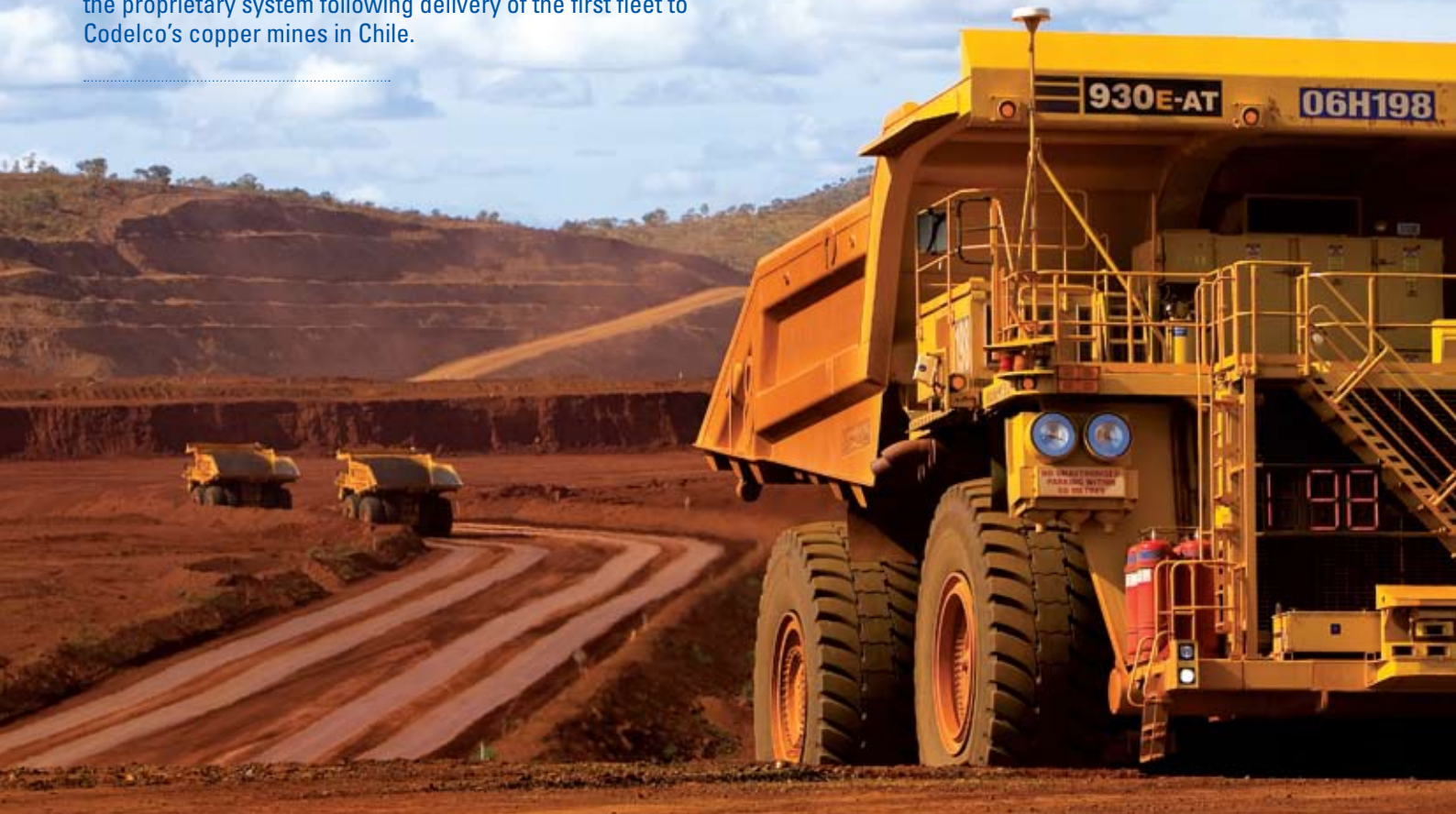
Above: Rio's West Angelas site operating Komatsu's autonomous 930E trucks loaded by the PC5500 (below).
