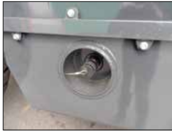
Fast Fuel System Wiggins flat face coupler for express fuelling.
