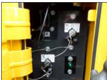
Lockable Battery & Starter Isolator Allow the machine to be isolated during maintenance tasks.
