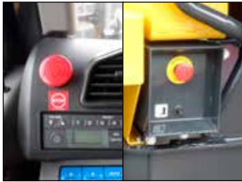
Emergency Stop 1 x Cabin 2 x External, provide machine shutdown in an emergency.
