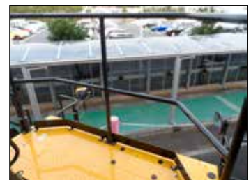
Handrail with 100 mm kickplate Provide safe access for both operators and maintenance staff.
