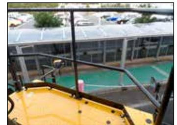
**Handrail with 100 mm kickplate**
