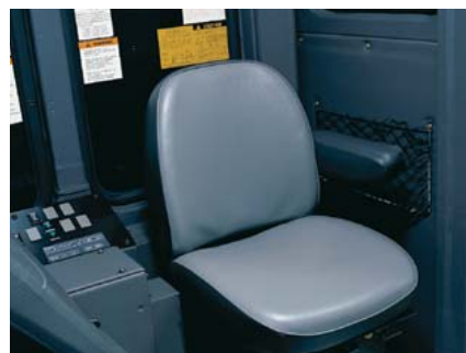
Auxiliary seat is provided as standard equipment; it is useful for on board training.
