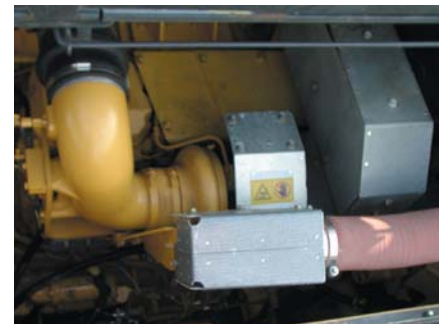
Thermal guards are placed around high-temperature parts of the engine and accessory drive.
