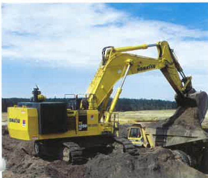
RTL's two PC1250-7 excavators are used for loading 50, 60 and 85 US ton dump trucks.
