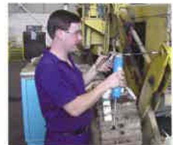
Now pump the grease into the cleaned joint until fresh grease starts exiting the joint. When you have finished, wipe off excess grease.
