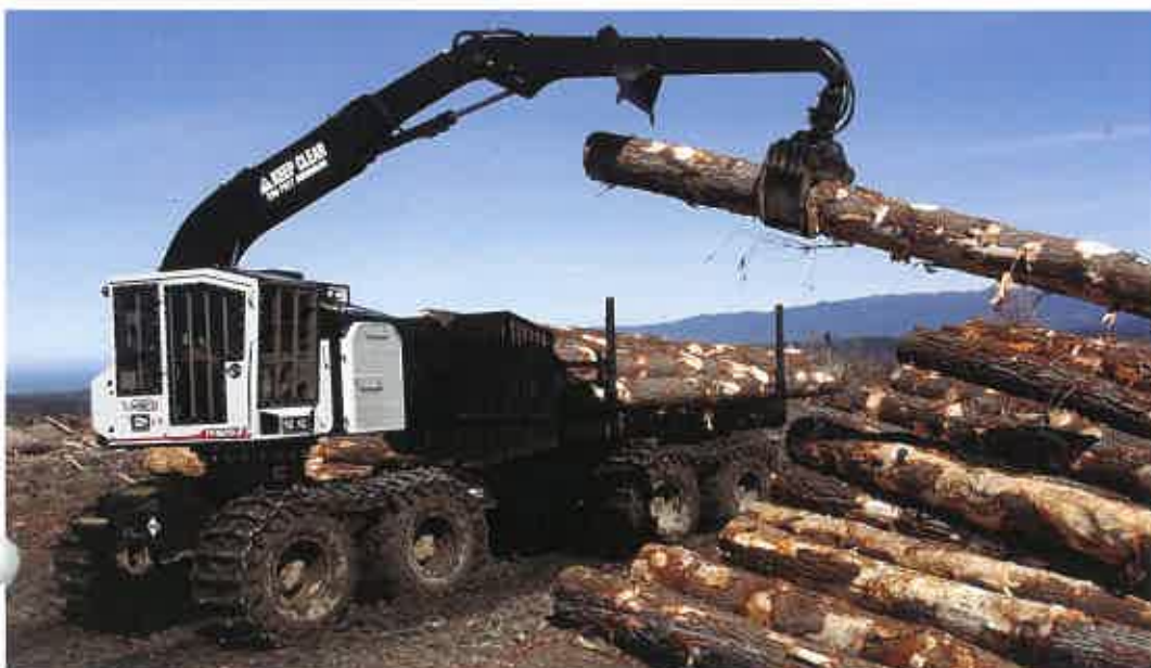
The 820E Forwarder loading logs at the DT King site in NZ South Island.
