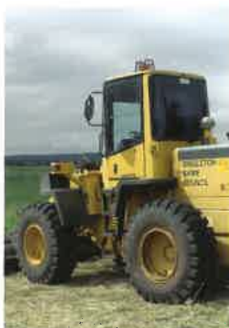
Singleton Council's WA180-3 wheel loader, fitted with 4:1 bucket.
