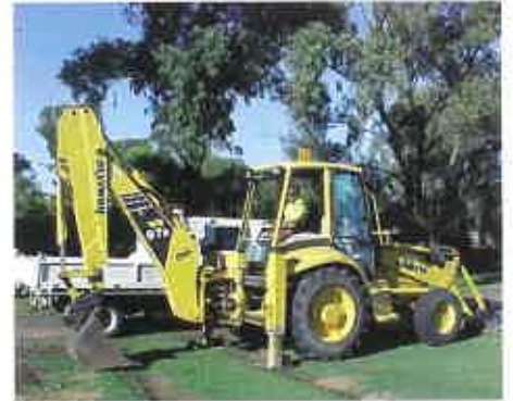
Dalby Town Council's Komatsu WB97R backhoe/loader, being operated by "Bud" Anderson, in the process of digging five grave sites, using a 750 mm bucket in very heavy black clay.
