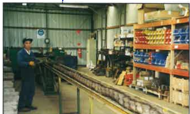
▲ Colin Lin, Track Press Operator overhauling a set of track chains.
