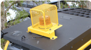
Rotating Amber Beacon Fitted with factory guard.
