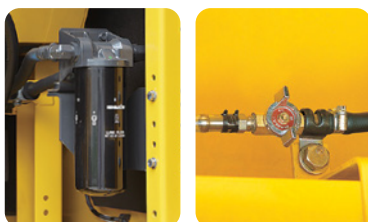
High efficiency fuel filter
