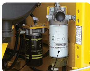
High efficiency fuel filter
