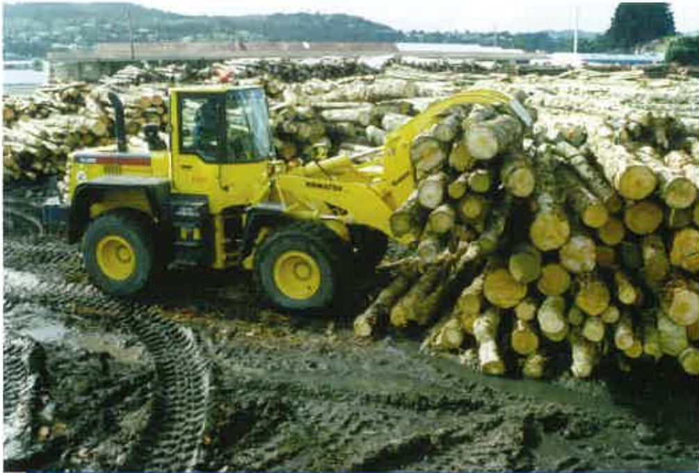
WA320-3 fitted with log grapples handling pulp logs
