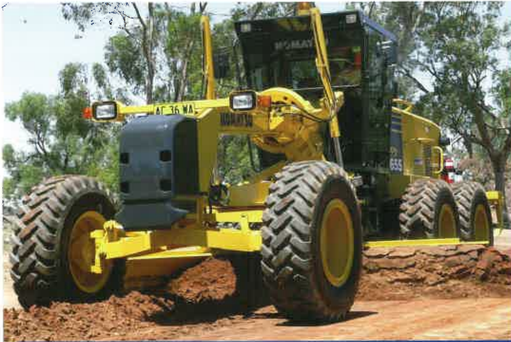
GD655-3 grader gives the operator great control for trimming work
