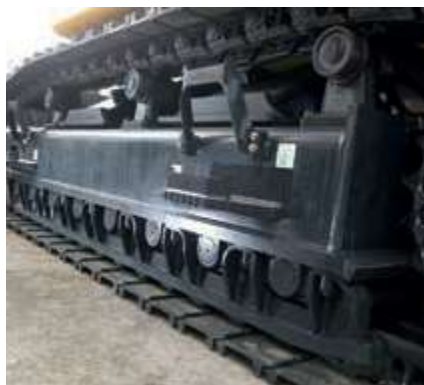
Full length track roller guards (optional)
