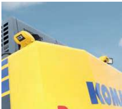
Rear-view and optional side-view camera
