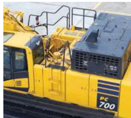
Hand rails and anti-slip plates
