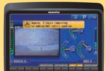
AdBlue® level and refill guidance
