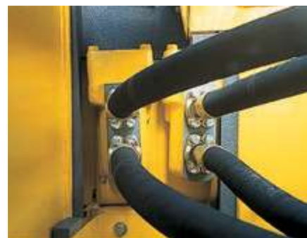
High pressure in-line filtration
