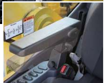
Armrest with simple height adjustment
