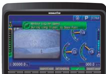
Eco-gauge, Eco guidance and fuel consumption gauge
