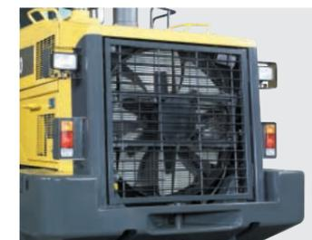
If the machine is operating in adverse conditions, the operator can reverse the hydraulic cooling fan from inside the cab by turning a switch on the control panel.
