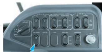
Dual mode engine power selection switch
