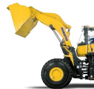
The WA500 enables loading onto 32t (40 Short ton) with the standard spec whereas WA500-6 necessitates the high lift boom with the 4.5m<sup>3</sup> bucket for it. Operator can get good visibility because of high his eye point.
