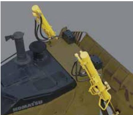
**Stroke sensing hydraulic cylinders**
