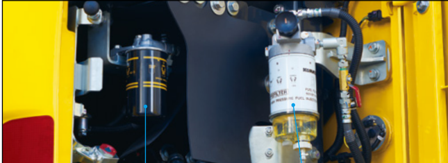
High efficiency fuel filter
