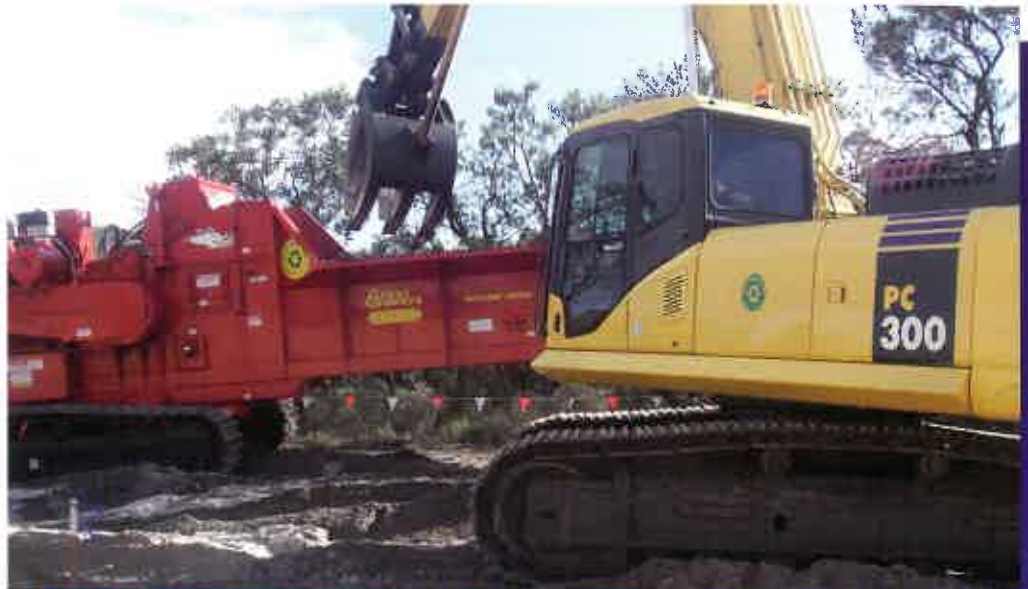
Grass Growers' PC300-7 fitted with grab feeding the company's purpose-built Woodhog 4600 grinder during work on WA's Roe Highway.
