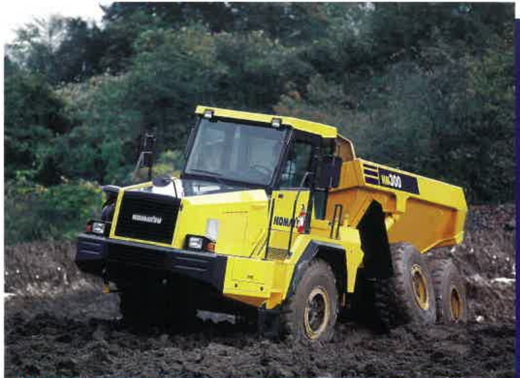
Komatsu's new 27 tonne HM300-1 articulated truck outspecs similar sized trucks on the market.
