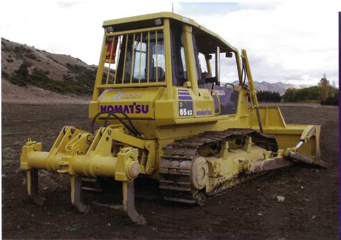
Costello Contracting's Komatsu D65EX-12 dozer; it's now done over 20,000 hours and still going well.
