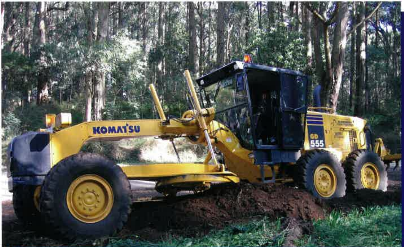
Murrindindi Shire's recently delivered GD555-3 grader at work on some of the shire's 400 km of unsealed roads.
