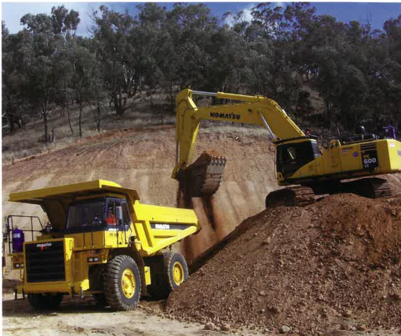
A PC600-7 excavator at Adelaide Brighton's Little Hartley Quarry loading a Komatsu HD325 dump truck.
