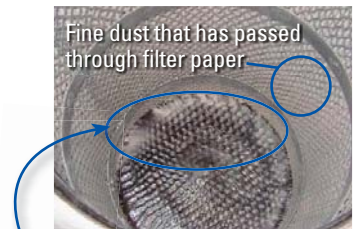
Non-Genuine Air Element Dust enters inside Air Element, due to faulty joint.
