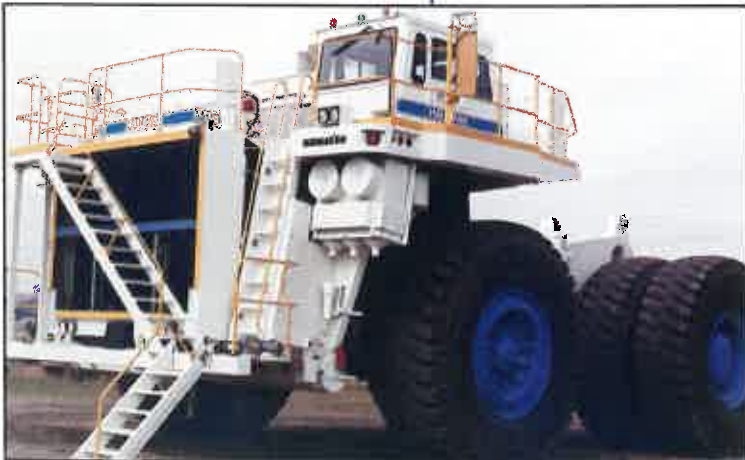
A Haulpak 830E truck less body awaiting delivery from Mt Thorley Branch, our Special Branch in this issue.
