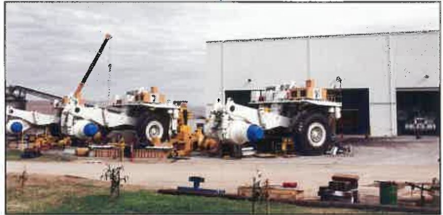
▲ Haulpak 830E's under assembly at Mt Thorley for R.W. Millers
